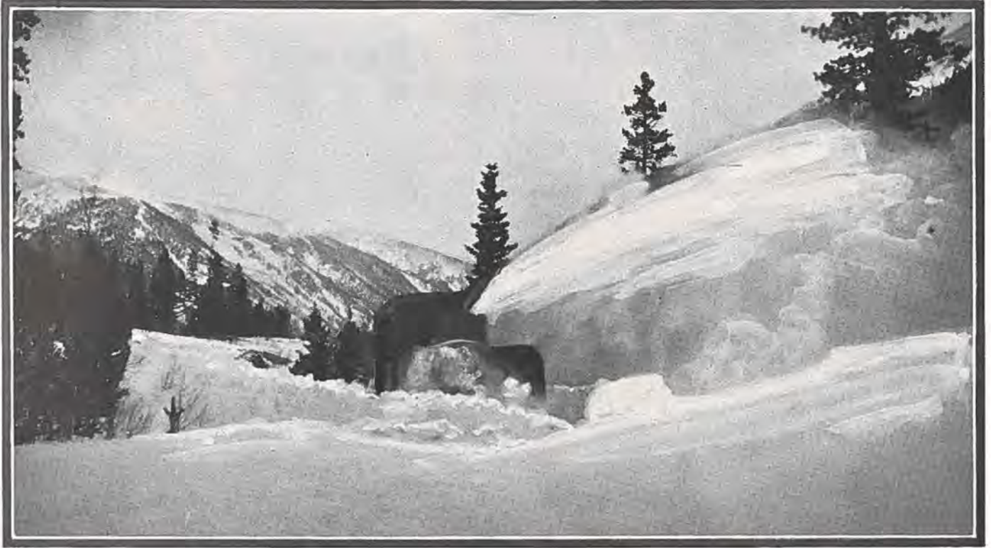
The highway department's new rotary snowplow working in 10 feet of snow and ice near the summit of Berthoud Pass.
