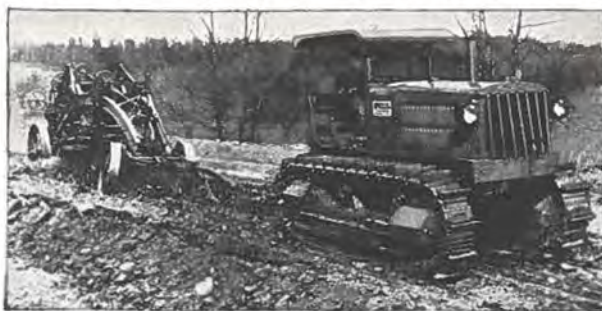
Monarch "50" pulling heavy 10-ft. grader with scarifier attachment in front of blade. Send for descriptive folders that give all details of the Monarch "50" and "75".
