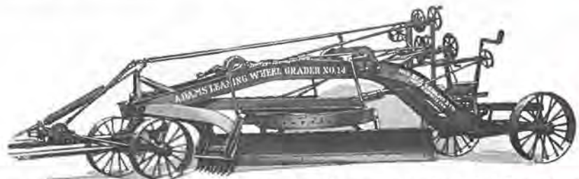
A new heavy blading machine recently placed on the market by the J. D. Adams Company.
